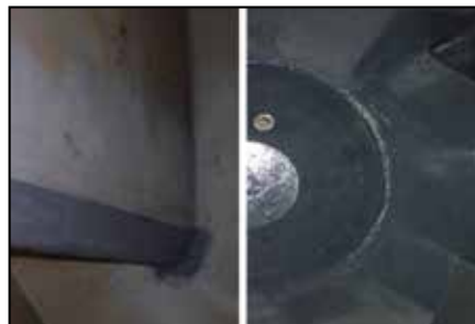
ARC BX2 applied to leading edge.
