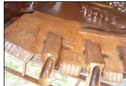
After 20 months only 5 kg of ARC BX1 was needed for repair.
